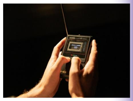
In place of the original display, I have installed and mounted a 1.3" OLED screen which displays preliminary onboarding text and graphics to represent the input data from the potentiometer. The displays are mounted with a custom fabricated part that I designed and 3D printed with recycled PLA.
